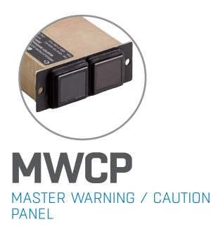
Master Warning / Caution Panel consists of two independent indicators for the annunciation to the pilot and copilot. Master Caution Rectangular Illuminated Indicator is responsible of indicating/resetting caution situations to pilot and copilot via illuminated buttons. Master Warning Rectangular Illuminated Indicator is responsible of indicating/resetting warning situations to pilot and copilot via illuminated buttons.
